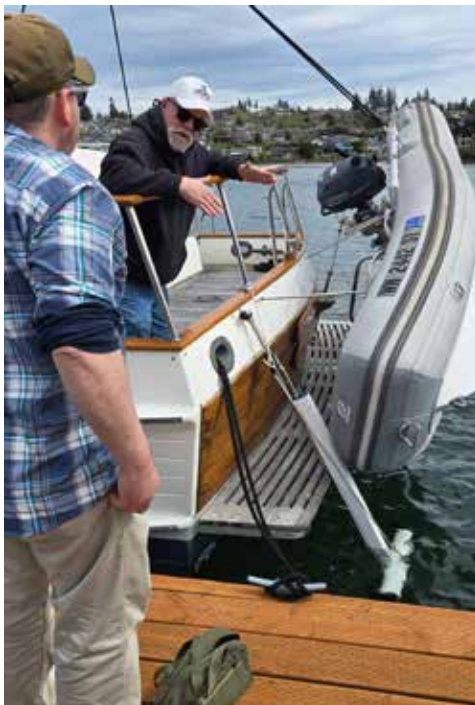
Tom Huebner helps a customer install a DockStar Smart Thruster, which mounts externally and requires no haul-out.
