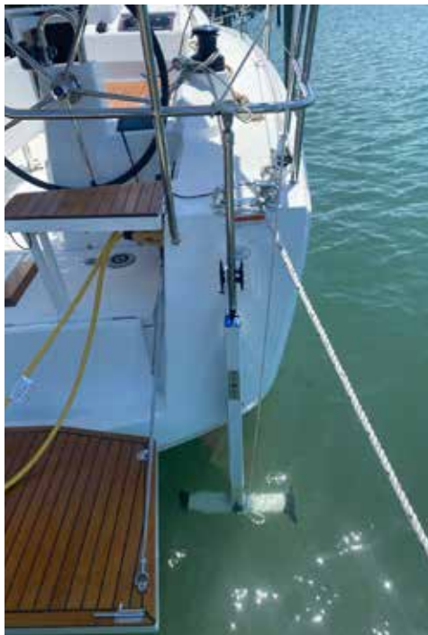
A DockStar Smart Thruster deployed on a Beneteau Oceanis 34 provides improved side-to-side maneuverability.
