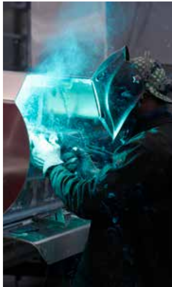
A SAFE Boats employee welds aluminum components as part of the boat-building process.
